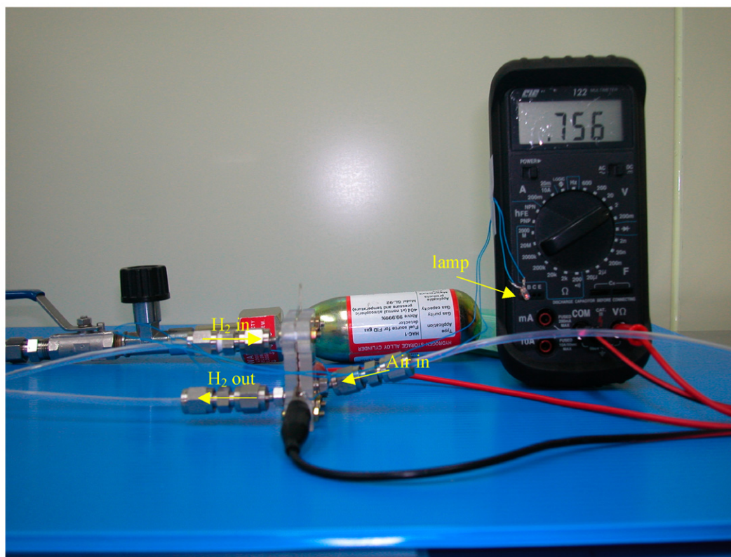
Fig. 2. Flow channel configurations and single fuel cell at operating condition: (a) the configurations of three flow channel and (b) interdigitated flow channel for single fuel cell.
